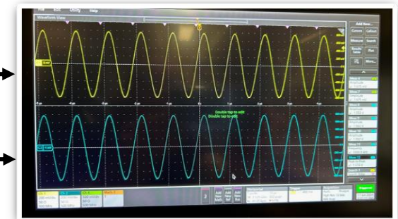
M00_AXIS = = 1MHz 1,6Vpp sur 50 Ohms M01_AXIS = = 1MHz 1,6Vpp sur 50 Ohms
